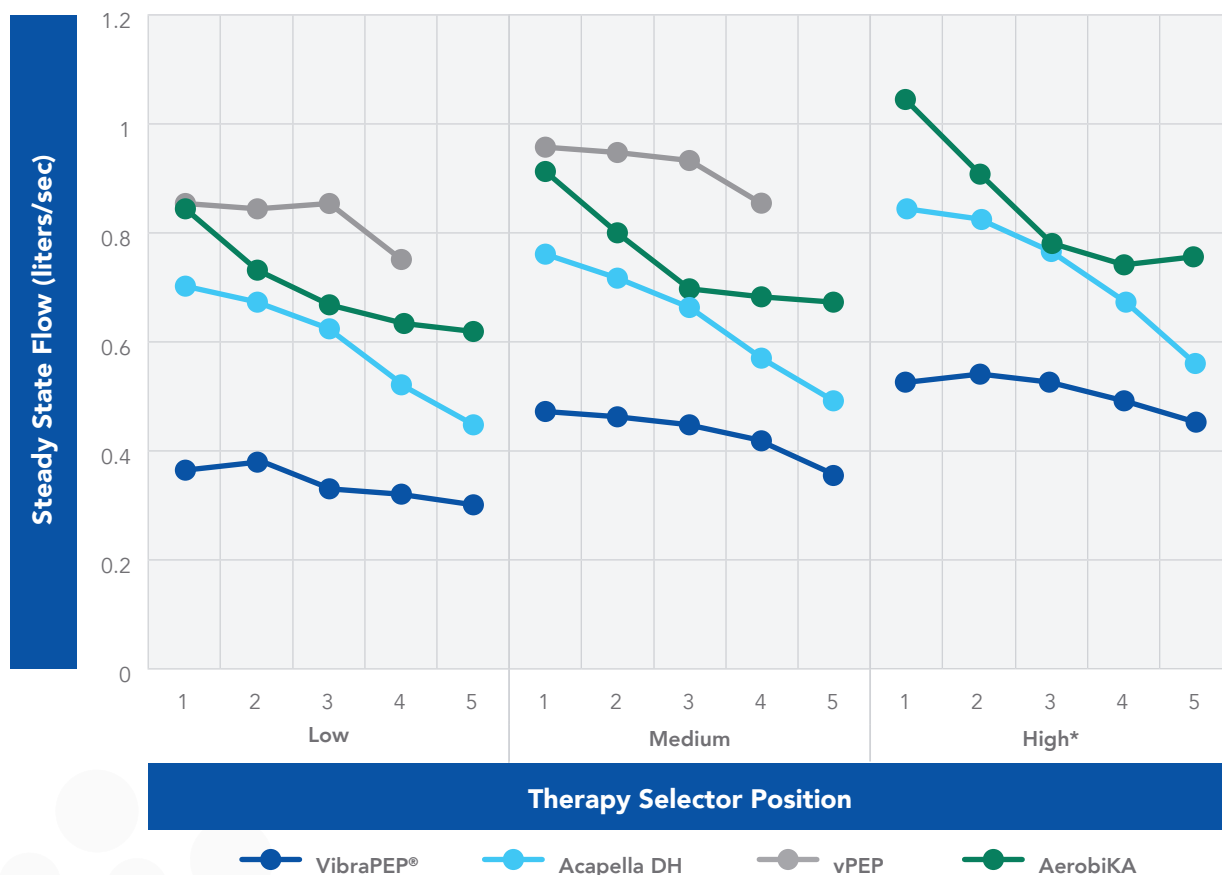
Steady state flow rates (liters/sec) for devices at the Low, Medium, and High target pressure. Error bars indicate 95% CI
